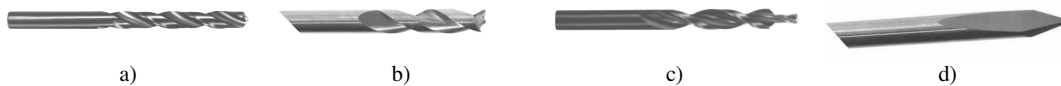
Figure 4. Drills considered in this work: a) twist; b) Brad; c) bi-diametric; d) Dagger.
