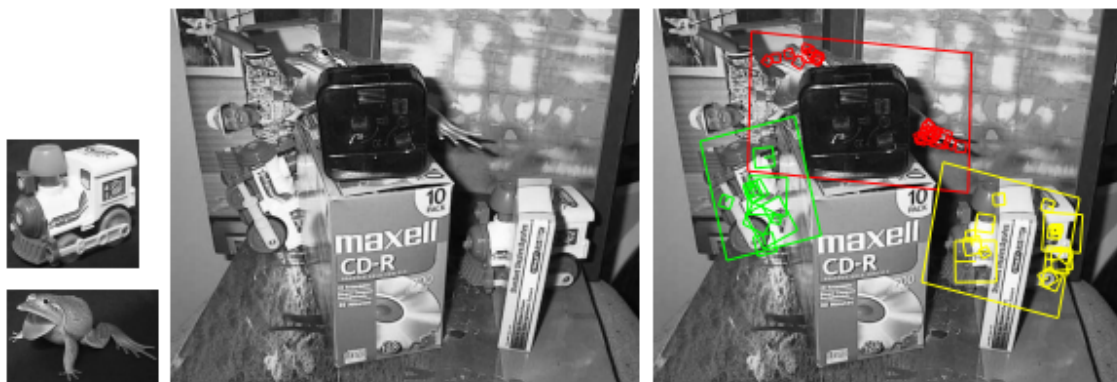
Figure 2.8: SIFT descriptor applied to an object matching problem. The objects are represented on the left images and the scene containing them on the right. The big squares represent the object match and the small squares the interest points detected. Extracted from [5].
