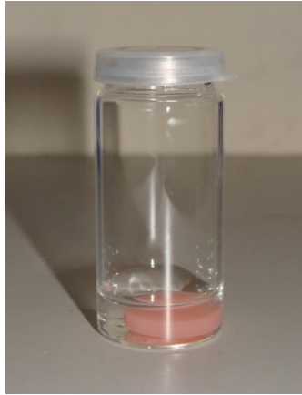
Fig. 6 – Acrylic resin sample submersed in artificial saliva inside a glass container (not opacified yet)
