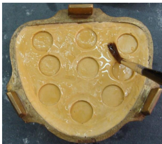
Fig. 3 – Gypsum isolation with separating fluid
