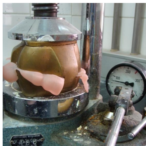
Fig. 5 – Flask loaded at 80 bar in hydraulic press
