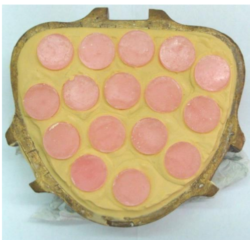
Fig. 2 – 3.0 x 15.0 mm wax patterns mounted in gypsum inside a conventional denture flask
