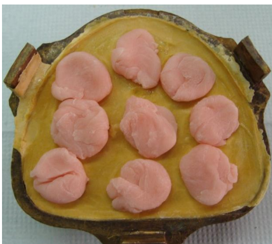
Fig. 4 – Covering of patterns with the polymer mass
