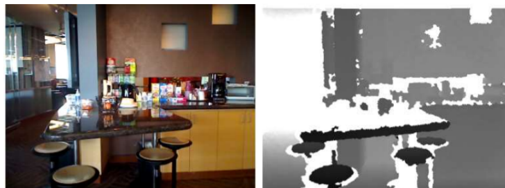
Figure 3.5: RGB image (left) and depth information capture (right) by an RGB-D camera. For the most part the white pixels in the right image means no depth value, due to occlusion, maximum distance, relative surface angle or material, (From [49])
