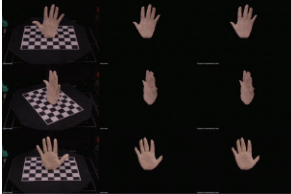
Figure 13. Three viewpoints (by row) of the 3D reconstruction obtained for the hand case. Left: original images. Middle: voxelized 3D model. Right: polygonized and smoothed 3D model.
