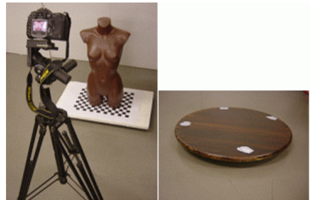
Figure 4. Left: camera and object layout. Right: simple turntable device used to reconstruct objects from images.
