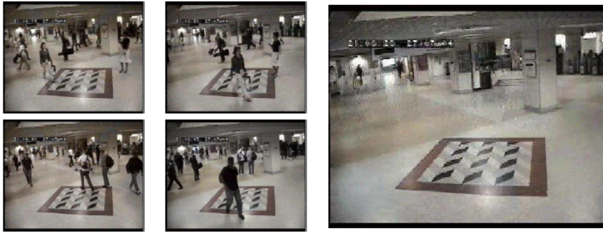
Figure 2.5: This image displays an effective background subtraction. Left:4 of the 20 input frames. Right: extracted background. Extracted from [51].
