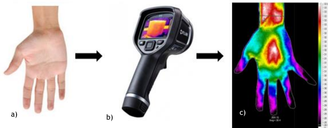
Figure 2.19 - Procedure for the production of a thermal image: a) Object; b) IR Camera Flir; c) Thermal image [88,89].
