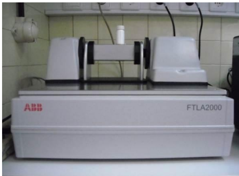
Figure 17: FT-NIR spectrometer FTLA2000 from ABB, equipped with a reflectance powder sampling accessory.
