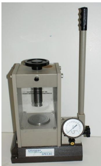
Figure 16: Hydraulic press used to produce tablets with variable hardness (adapted from (89)).
