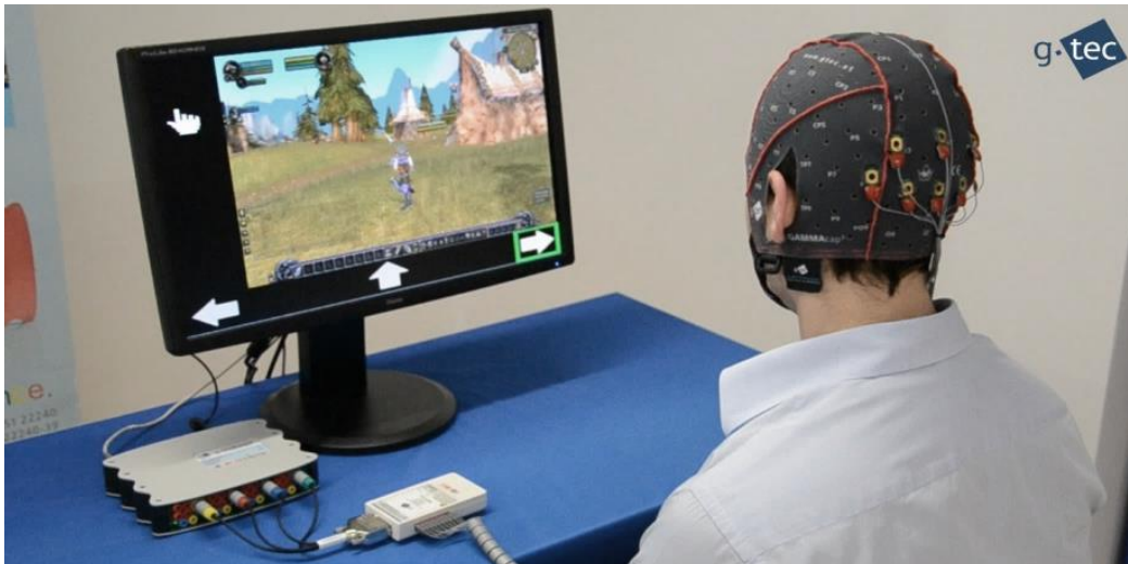
Figure 59. The brain-computer interface enables the playing of computer games with one's thoughts, presentation of the application called "SOCl" - Screen-Overlay Control Interface (intendiX, n.d.)
