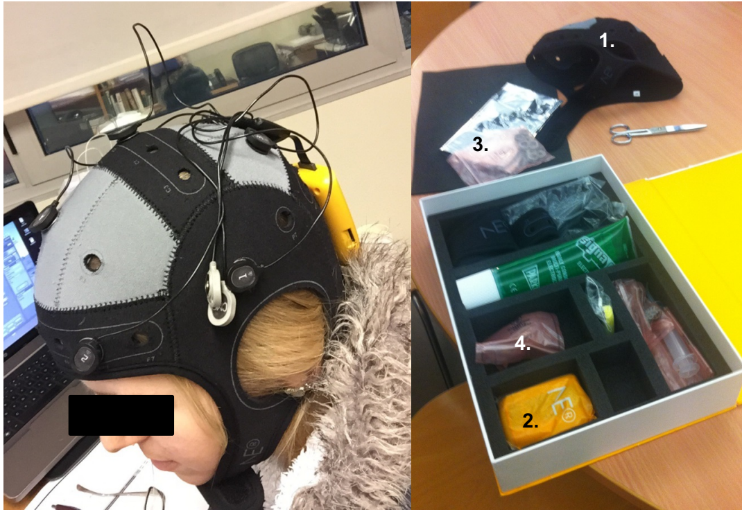
Figure 72. Enobio 8 Neoprane headcap, with installed 8 dry electrodes (left) and the EEG data acquisition kit including 1. Washable cap; 2. Battery with bluetooth emitter; 3. Set of 8 dry electrodes; 4. Cables. (photos by author).
