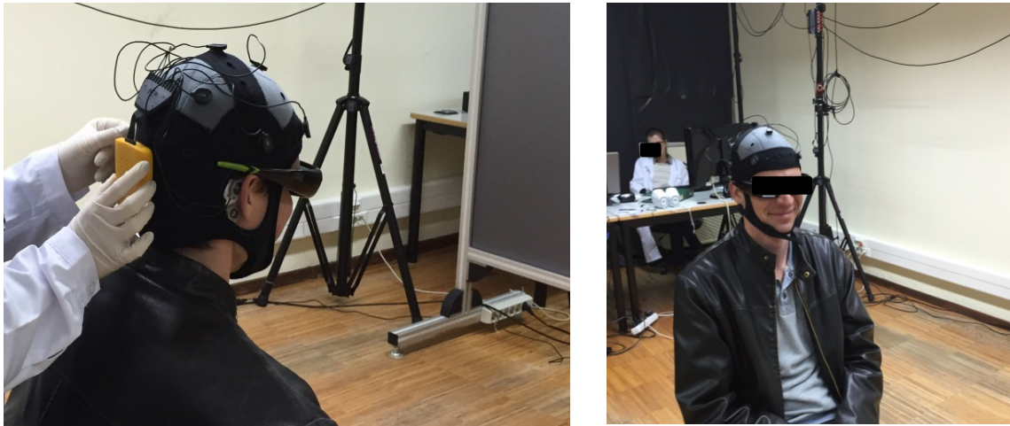
Figure 74. A participant with Enobio device and 3D shutter glasses installed. On the left: turning on the Enobio connecting device, on the right: participant ready for the data collection.
