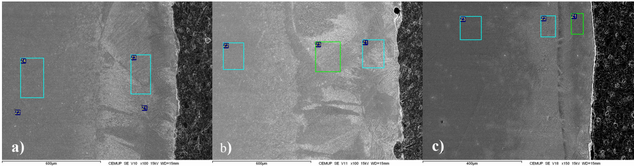
Fig. 5 Microstructure of Ti10V2Fe3Al alloy casted in ceramic moulds of: a) ZrO_2-Y_2O_3 , b) ZrO_2-CaO and c) Y_2O_3 .
