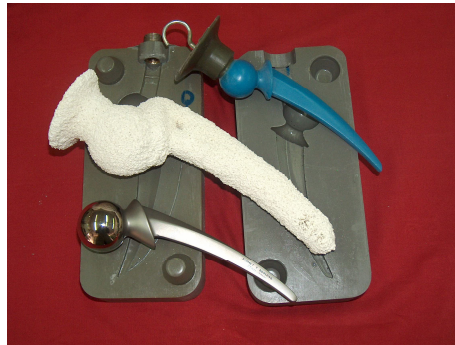
Fig. 2 From the top to down: Wax pattern with the pouring system, ceramic shell and Ti casted part placed over the composite mould used to inject the wax model.
