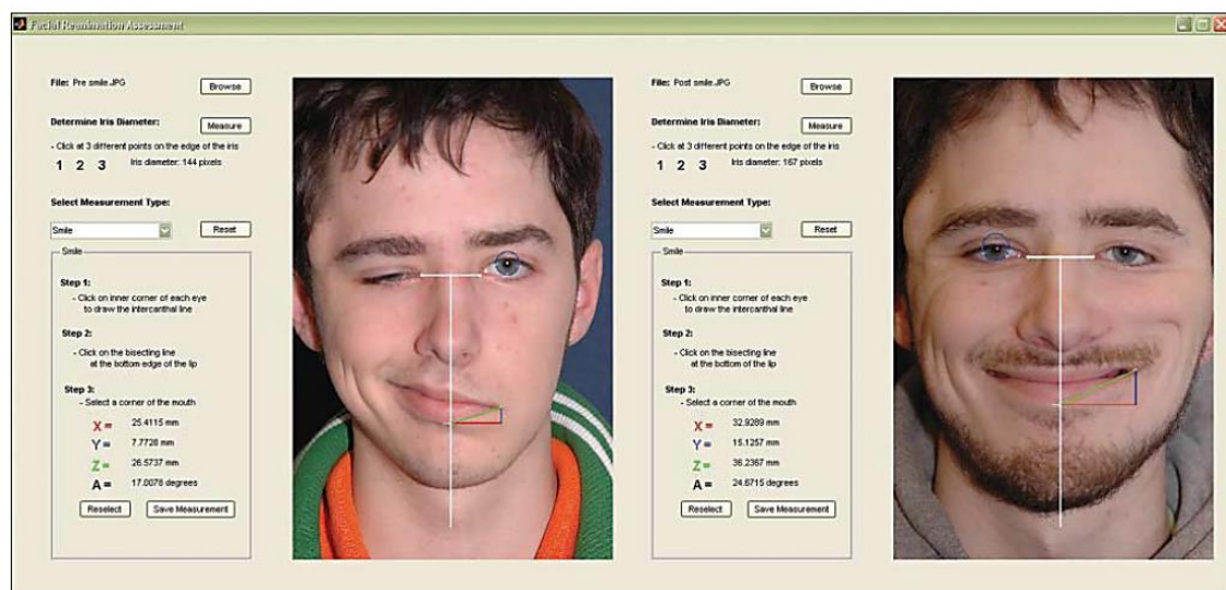
Figure 7. Preliminary SMILE interface (implemented in MATLAB software), for measurement of lip excursion during smiling. Retrieved from [57].
