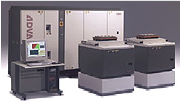
Figure 1: A typical automatic production test station for modern SDRAM devices.
