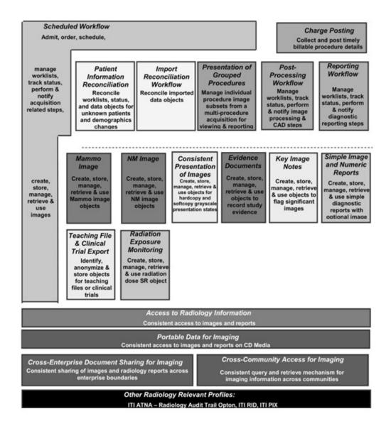
Figure 3.5: Representation of the different Workflow Profiles from the IHE Radiology Domain. Taken from Technical Framework Volume 1 (IHE RAD TF-1).
