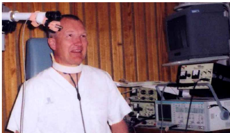
Figure 2.5. EGG measurement setting. Electrodes have been placed on the subject's skin and a band has been adjusted around the neck to hold the electrodes in place. The electroglottograph (Glottal Enterprises MC2-1) is on the right on top of the oscilloscope [Pul05].
