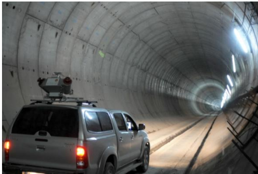
Figure 2. Riegl VMX-250-CS6 mobile laser scanning system in operation in a tunnel survey.
