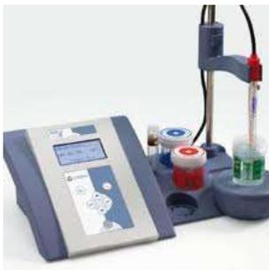
Figura 11 - *Basic 20 pH-meter* (*Crison Instruments S.A., Spain*)<sup>37</sup>
