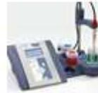
Basic 20 pH-meter, Orion instruments, Spain
