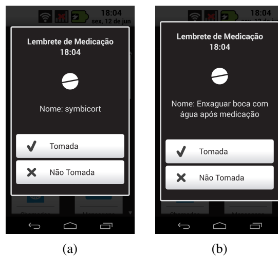
Figure 4.8: Illustrative example of the medication reminder: (a) shows the alarm to remind the patient to take the medication and (b) alerts the patient to rinse the mouth with water in case of medication intake with corticosteroids.
