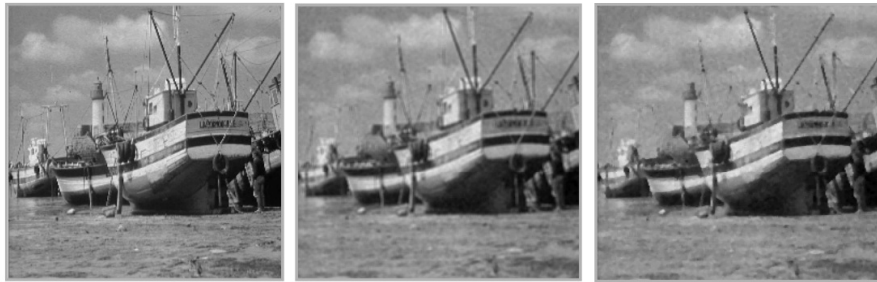
Figure 2.1: Result of the application of a Gaussian filter (middle) and median filter (right). Original image on the left [1]
