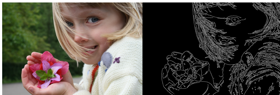
Figure 2.2: Result of the application of the Canny edge detector [1]
