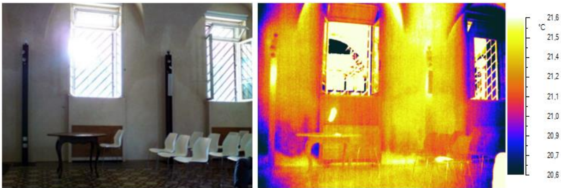
Fig 4.19 – Visual picture of the southeast wall, between 3 rd and 4 th window, (left) and correspondent thermogram from the survey of September 9 th , 2015 (right)
