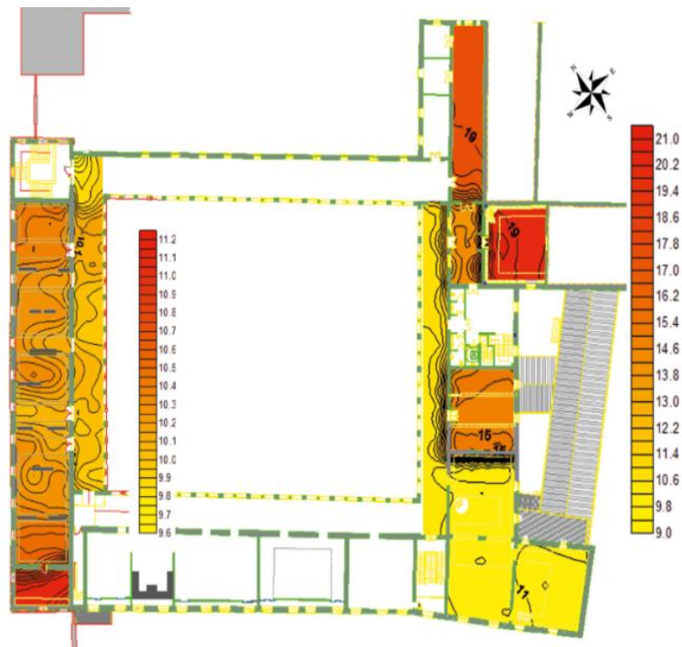
Fig 4.29 – First floor Temperature map from the 9.30h measure, from the February 4 th , 2015, survey.
