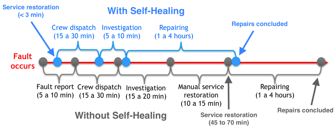
Figure 2.5 - Comparison of response time between a Self-Healing capable network and a conventional network [10].
