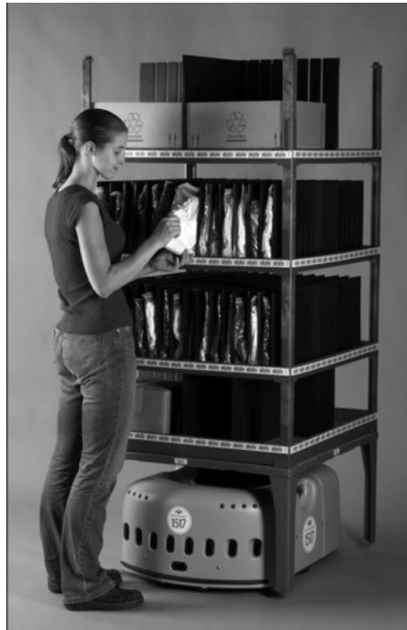
Figure 1.1: A Kiva Drive Unit and Storage Pod [4].
