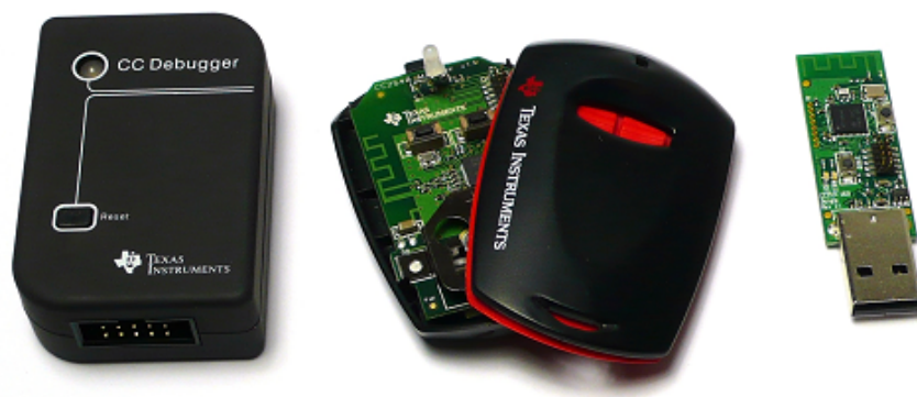
Figure 3.3: Bracelct Prototype - CC2540 module from Texas Instruments
