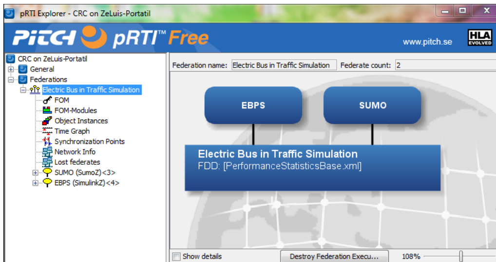
Figure 6.1: Pitch pRTI GUI with connected federates
