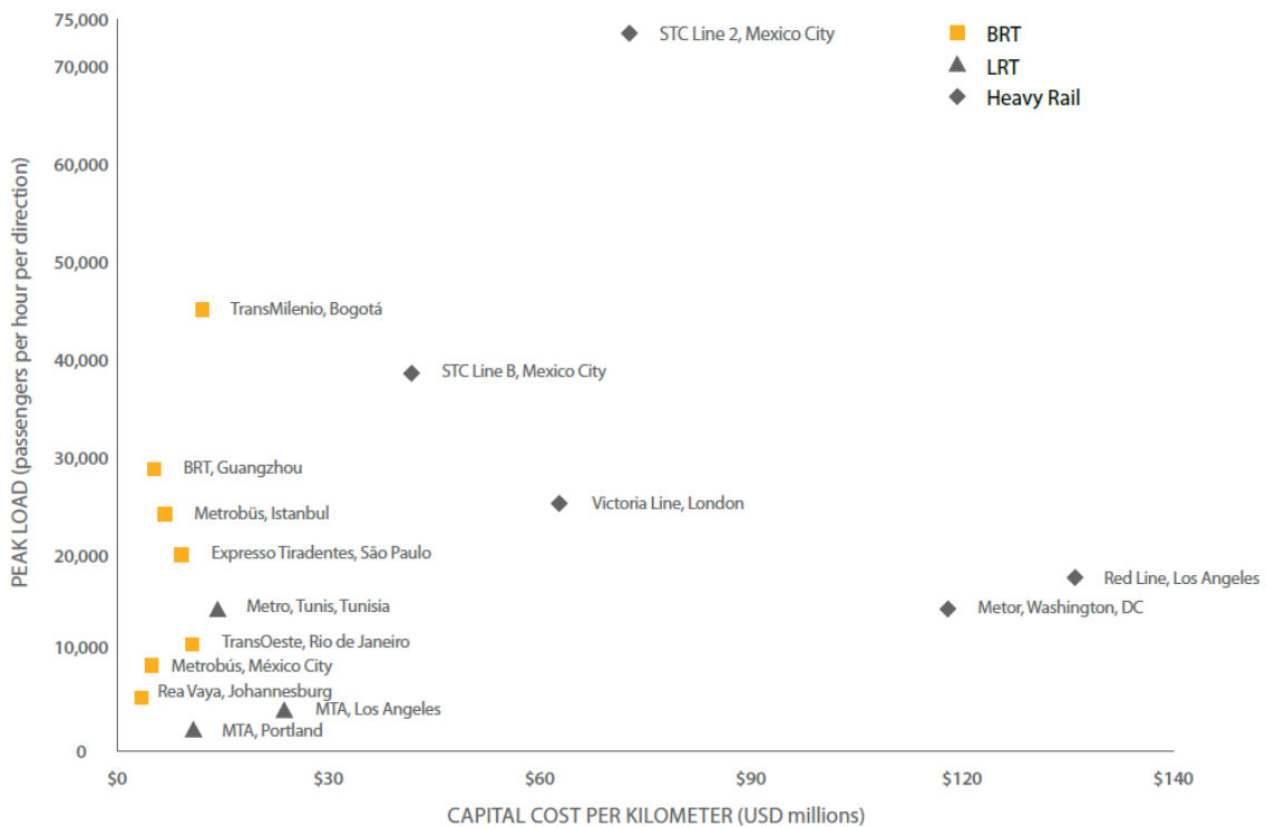
Fig.3.16 - Comparison of capital costs and peak loads of some transit systems (EMBARQ, 2013) [22]
