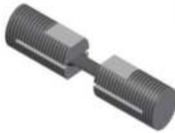
Figure 4.21: Adhesively bonded specimen to threaded metallic endcaps [128]
