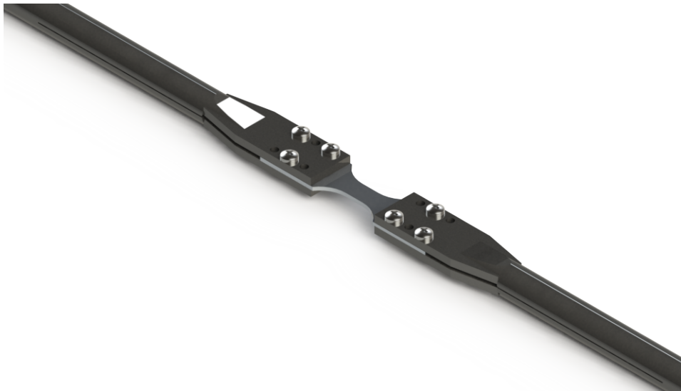
Figure 4.22: Gripping system which uses screws to fix specimens with respective holes
