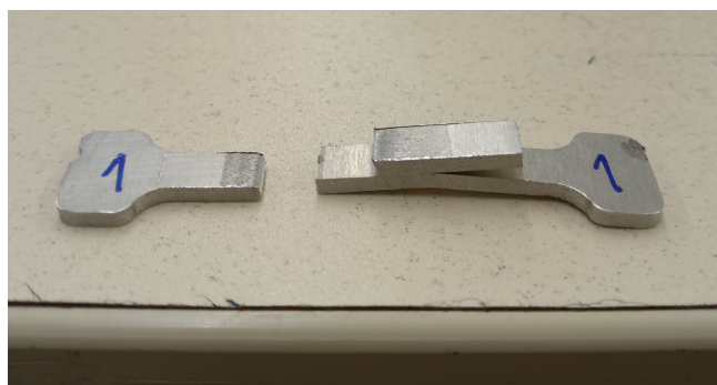
Figure 5.37: Overlap specimen rupture
