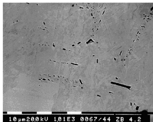
Fig. 5. Microstructure (1000×) after 336 h of annealing (overall composition: w(\text{Zn}) \sim 0.3 and w(\text{Bi}) \sim 99.7\% ). The matrix comprises a solid solution of Zn in (Bi) phase and dark particles formed by a solid solution of Bi in (Zn).
