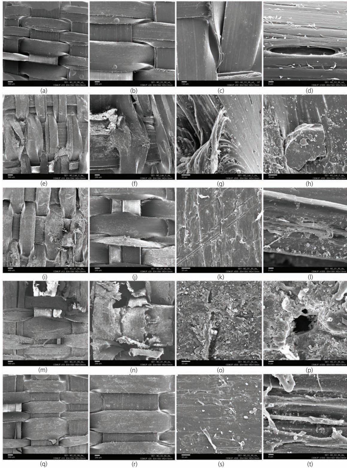
Figure 3. SEM images of geotextile GTX2: intact (INT) — (a) \times 10 , (b) \times 20 , (c) \times 500 , (d) \times 1000 ; damaged in laboratory (ID LAB) — (e) \times 10 , (f) \times 20 , (g) \times 500 , (h) \times 500 ; installed in soil 1 compacted to compaction energy 1 (ID-S1-CE1) — (i) \times 12 , (j) \times 20 , (k) \times 500 ,
