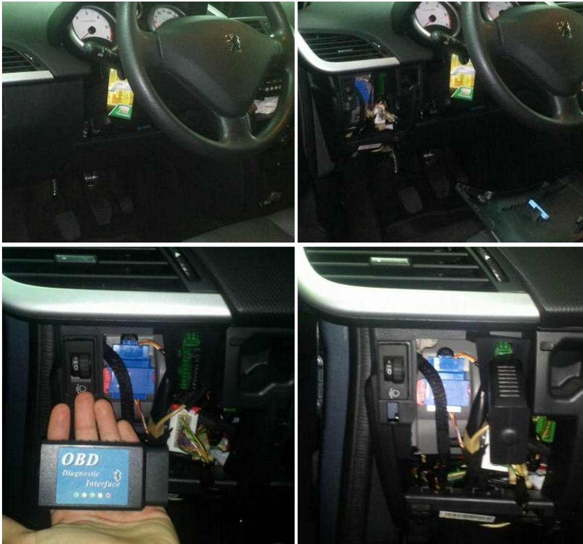
Figure 5.3: Mounting an OBD device to a Peugeot 207
