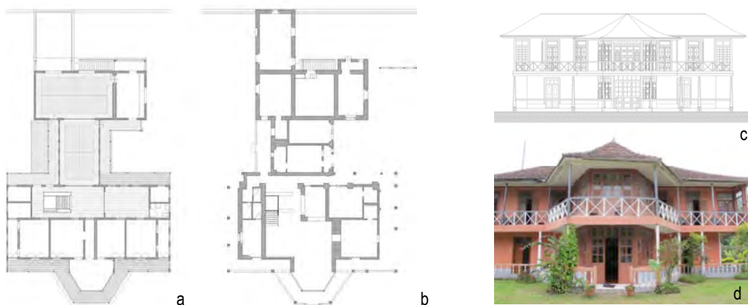
Figure 12. Example of on-going architectonic survey, main house, Roça Bombaim, São Tomé – (a) plan of the first floor, (b) plan of the ground floor, (c) front elevation, (d) photograph [ASF+HMS].
