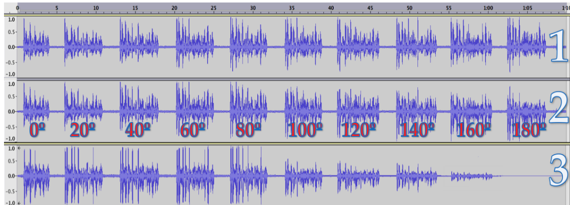
Figure 4.13 - 1-Left input 2-Right input with signals out of phase from left input 3-Output from the FPGA after signal inverter for angle control.
