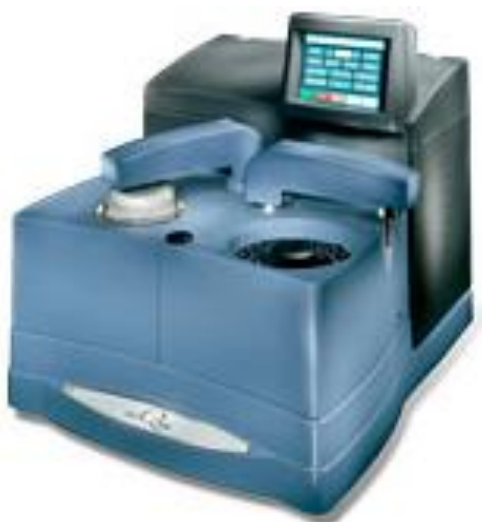
Figure 1.3 - The TA Instruments Q1000 used in this work for phase transitions measurements.
