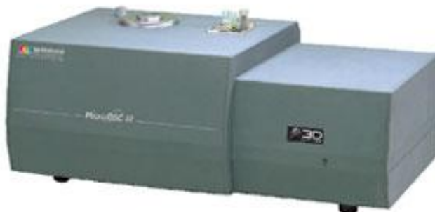
Figure 1.5 - The Setaram \mu DSC IIIa used in this work for heat capacities measurements.
