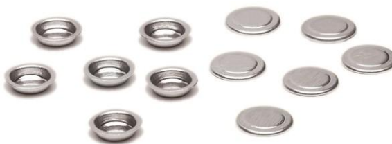
Figure 1.4 – The 10 mm 3 Tzero series hermetic pans used in the TA Instruments Q1000.
