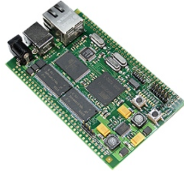
Fig. 1: The ICnova AP7000 Base board (9,65 x 6,1 cm)
