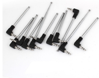
(a) The Si4703 FM Tuner Evaluation board [44]. (b) The telescopic antennas used with the FM Tuner board, to improve the RDS reception.
