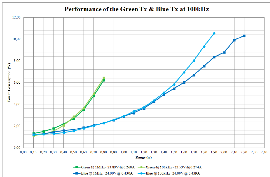
Figure 4.14: Test results using different transmission frequencies of 100kHz and 1MHz.
