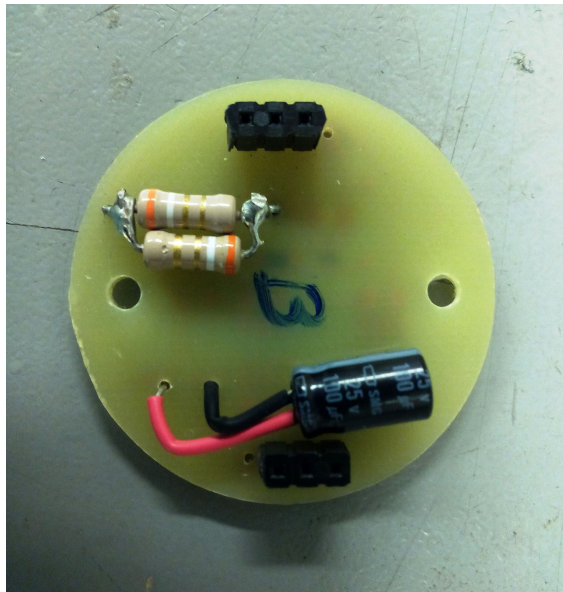
Figure 3.40: The improvised capacitor in the primary prototype.
