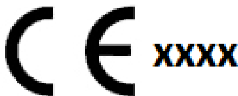
Figure 2.5: Example of the CE mark; "xxxx" represents the four digit number attributed to the notified body.
