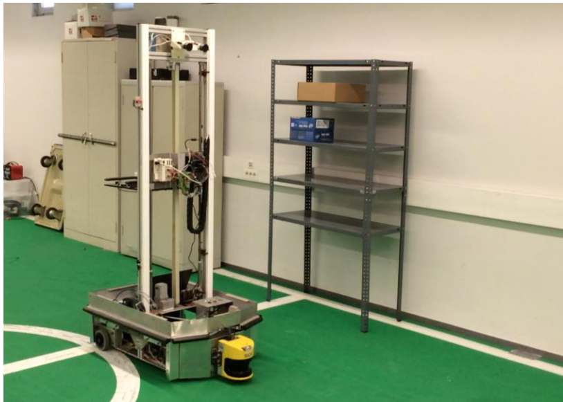
Figure 41 - Mobile Robot Acquiring Point Cloud data.
