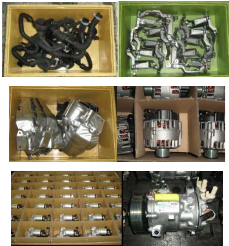
Figure 4 - Engine pipe, engine support, thermal shield, alternator, starter and air conditioning compressor, respectively [5].
