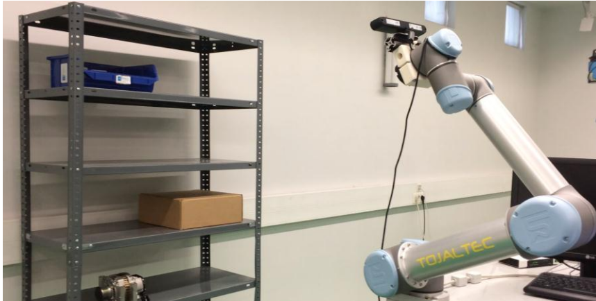
Figure 35 - Acquisition Scenario 1. The UR5 Robotic Arm performs several movements, always remaining fixed on an unmoving table.
