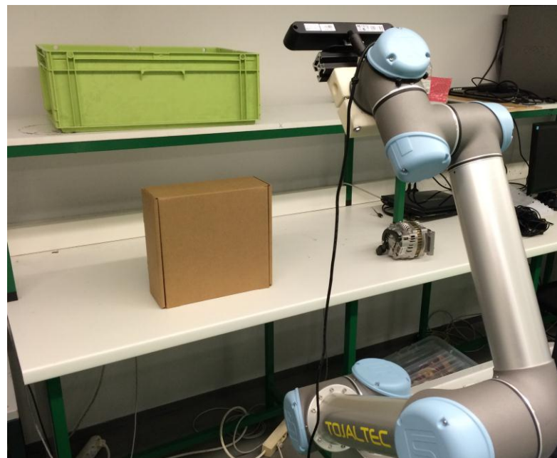
Figure 32 - Camera Calibration Process, phase 2. Example of robot position.
