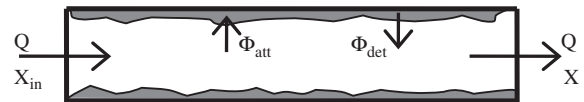
Fig. 2 – Bulk water cell balance in the reactor system. ( \Phi_{att} —rate of cell attachment; \Phi_{det} —rate of cell detachment from the surface; Q —water flow rate; X_{in} —inlet water cell density; X —outlet water cell density (= reactor bulk water cell density, assuming a perfectly mixed system).
