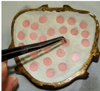
Fig. 1 – Modeling wax calibrated circular patterns used for the fabrication of the samples by compression molding technique.
