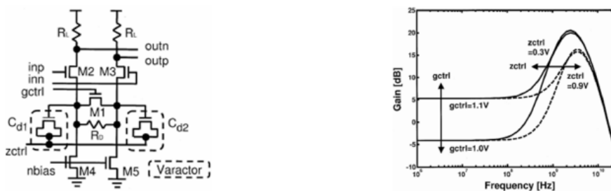
Figure 2.13: Equalizer Schematic reprinted from [9] Figure 2.14: Equalizer Transfer Function reprinted from [9]
