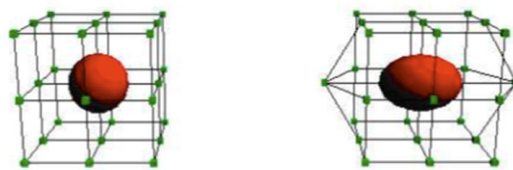
Figure 2.5: Free-Form Deformation applied to a spheric surface: controlling box and embedded object; left: neutral position; right: object deformation [1].
