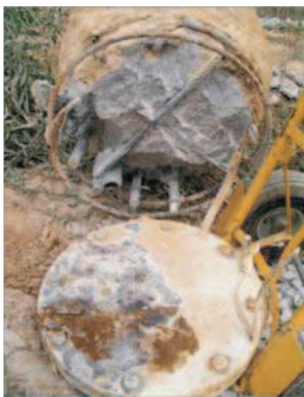
Figure 24 - Load cell and the pile base (Costa Esteves, 2005).
