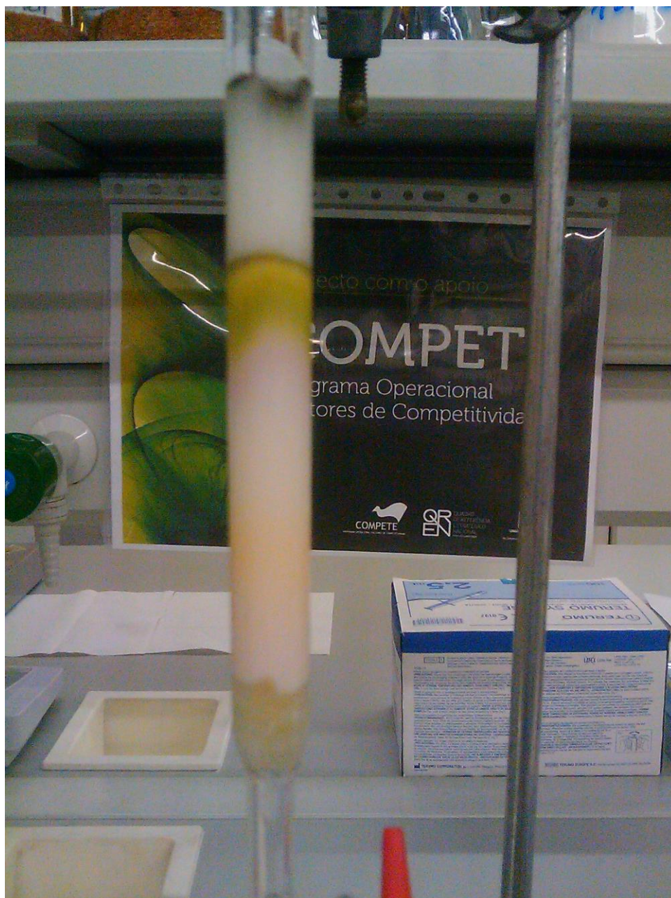
Figure C.5. 1 – Alumina column (SPE) after sample loading ( Pinus pinaster needles) and elution with 50 mL DCM/Hex (1:1)
