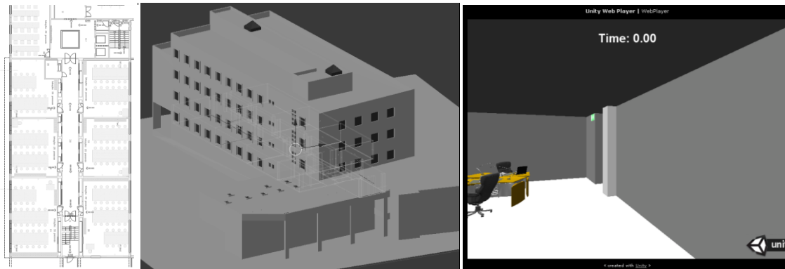
Figure 4.4 – FEUP “I” building 1st floor architectural blueprint (2D), 3D model in Blender and 3D rendered view of the building in Unity3D showing LIACC lab I121
