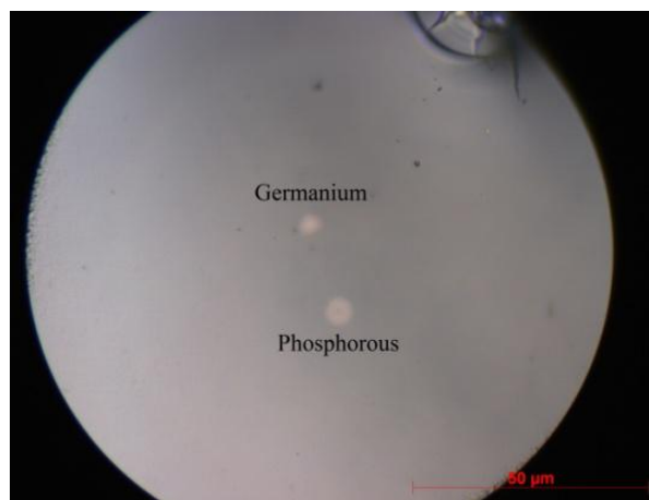
Fig. 6.5 Cross-section of the dual-core fibre, showing the germanium and phosphorous doped cores.
