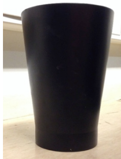
Figure 6.4 - Dark cone with a diameter between 80 and 130.5 mm, used for the system characterization tests.
