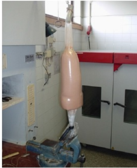
Figure 2.15 - Finishing the final socket with a termoplastic material [13].
