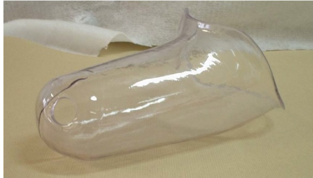
Figure 2.13 - Socket prototype in polypropylene [13].
