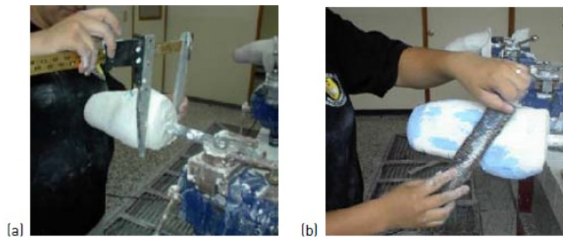
Figure 2.11 - (a) Dimensional verification of the stump replica [13].
