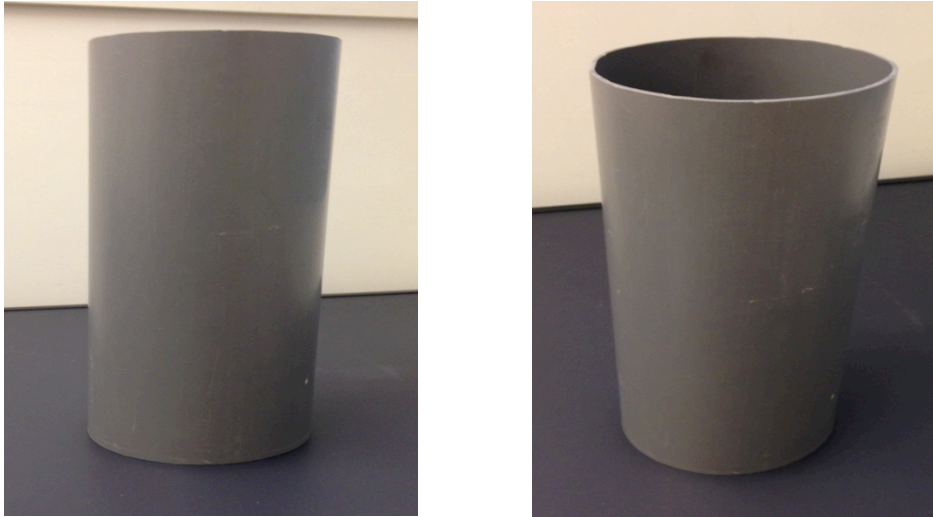
Figure 7.1 - Photos from two different views of the PVC dark grey tube with 121.2 mm diameter that was used in the scanning experiments.
