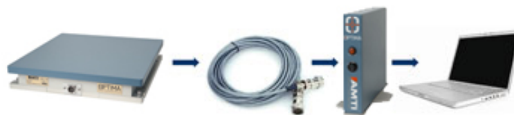
Figure 5 - Force plate components (AMTI 2013)
