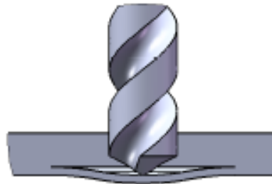
Figure 1: Delamination mechanism: the last material ply is separated from adjacent ones.
