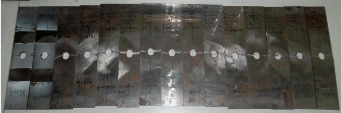
Figure 6.9 – Specimen plates made of puddle iron from the Eiffel bridge with a circular hole (dimensions in mm).
