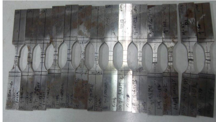
Figure 3.10 – Some smooth specimens of material from Eiffel bridge used in fatigue tests.
