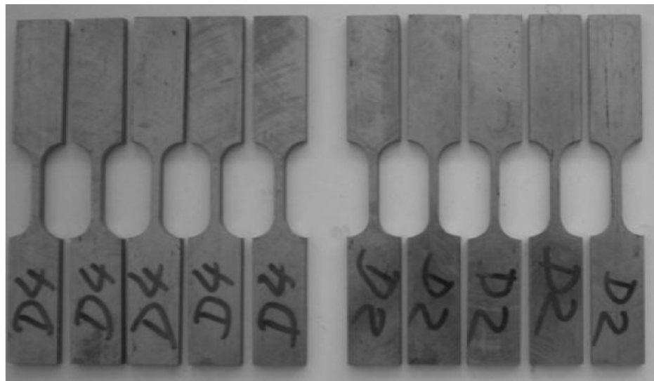
Figure 3.11 – Some smooth specimens of material from Fão bridge used in fatigue tests [13].
