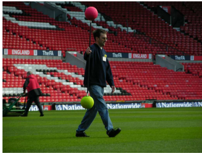
Figure 2.4: A wand-like calibration object with two balls of different colours. From [26].
