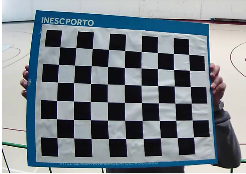
Figure 4.1: The calibration pattern used was a 9 \times 6 chessboard pattern, with a square size of 5.4 centimeters. The calibration pattern was moved around the camera's field of view, exploring as much as different orientations to improve the intrinsic parameters estimation.
