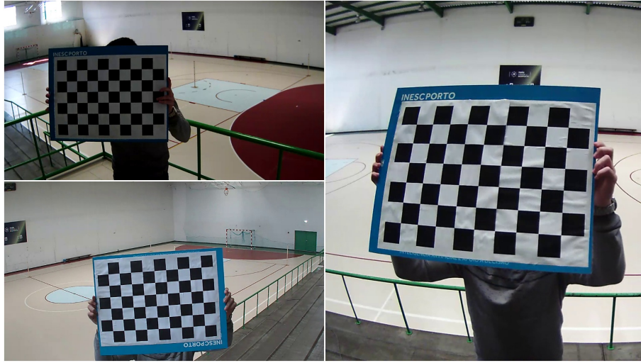
Figure 3.9: One frame example from three of the four installed cameras, displaying the used calibration pattern. To produce better results, the pattern was rotated and moved with several orientations in front of the cameras so that several frames with different pattern positions could be identified, thus detecting the corners from the black and white chessboard with differentiated poses.
