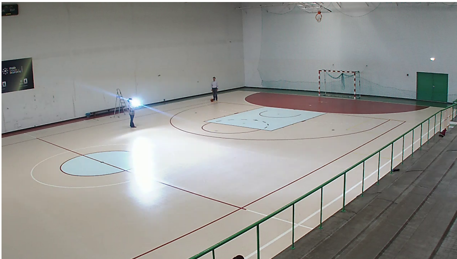
Figure 3.5: One view of camera IP4. An electronic flash device produced a bright light allowing to synchronize all cameras for the ball in continuous motion sequences.
