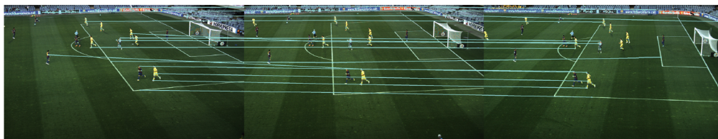
Figure 2.8: Multicamera feature matches, considered as inliers. Most outliers are removed using the angle-based filtering. Only a subset of the multicamera matches are shown. From [58].
