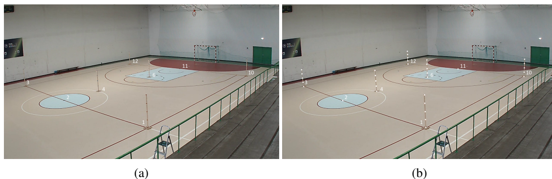
Figure 4.4: One view of camera IP4. (a) 6 markers, with 5 different heights labelled with red duct tape, distributed around the basketball field. Those points, plus two others from the baseline and the center line, formed the 32 3D world points used to estimate the pose of the camera, a value that depended on the number of points observable from each camera. (b) White dots represent the projected points estimated using the Iterative solution; they must coincide with the image of the 3D world points defined on the markers and on the field.
