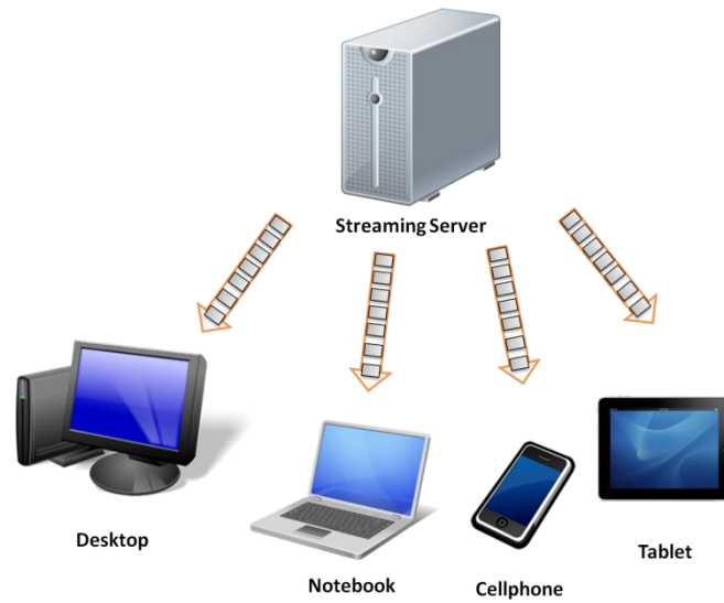
Figure 6 - Server-Client system using a progressive download protocol.
